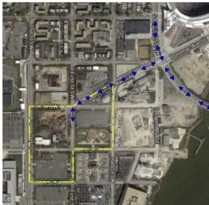
Figure 5.3: Construction Traffic Management Plan (Illustrative Only)
