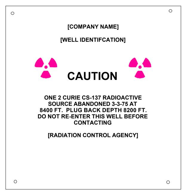
The size of the plaque should be convenient for use on active or inactive wells, e.g., a 7-inch square. Letter size of the word "CAUTION" should be approximately twice the letter size of the rest of the information, e.g., 1/2-inch and 1/4-inch letter size, respectively.
